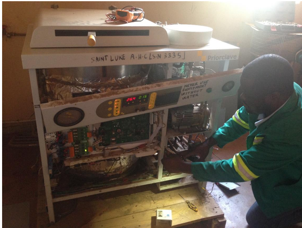
Mr. Hiram Kalumbi repairing the autoclave at Msoro Clinic.
